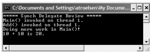
Figure 14-1. Synchronous method invocations are “blocking” calls.
